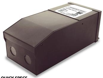
KLUS - MD-300-12 is the most compact LED driver on the market with a magnetic transformer core. It is equipped with two push-to-reset circuit breakers on the input and output, which protect both the load and driver. The driver is encased in a coated metal box that includes 2 knock-outs on the bottom to enable easy installation that complies with electrical code requirements.
